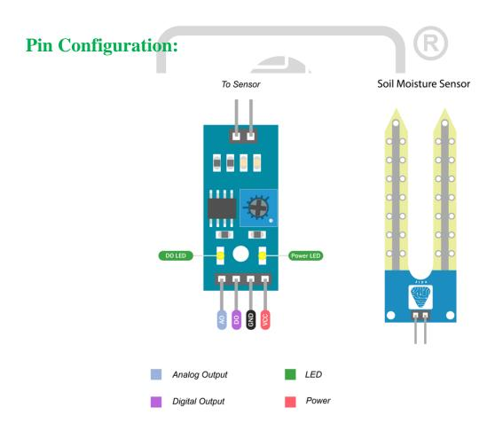
VCC: supplies power to the sensor. It is recommended that the sensor be powered from 3.3V to 5V. Please keep in mind that the analog output will vary depending on the voltage supplied to the sensor.
